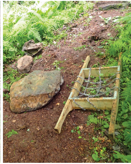
From left: Tyler installing bridge decking; Seasonal Trail Crew staff bench cutting new trail and building water bars; Ernie the Gurney is a two person rock carrier, built by Tyler.
